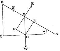
The body is maintained in equilibrium by the three forces P, W, R, and the directions of these forces are respectively parallel to the sides of the triangle EGD; therefore, by the triangle of forces,
